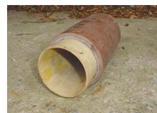
Liner inside clay pipe
